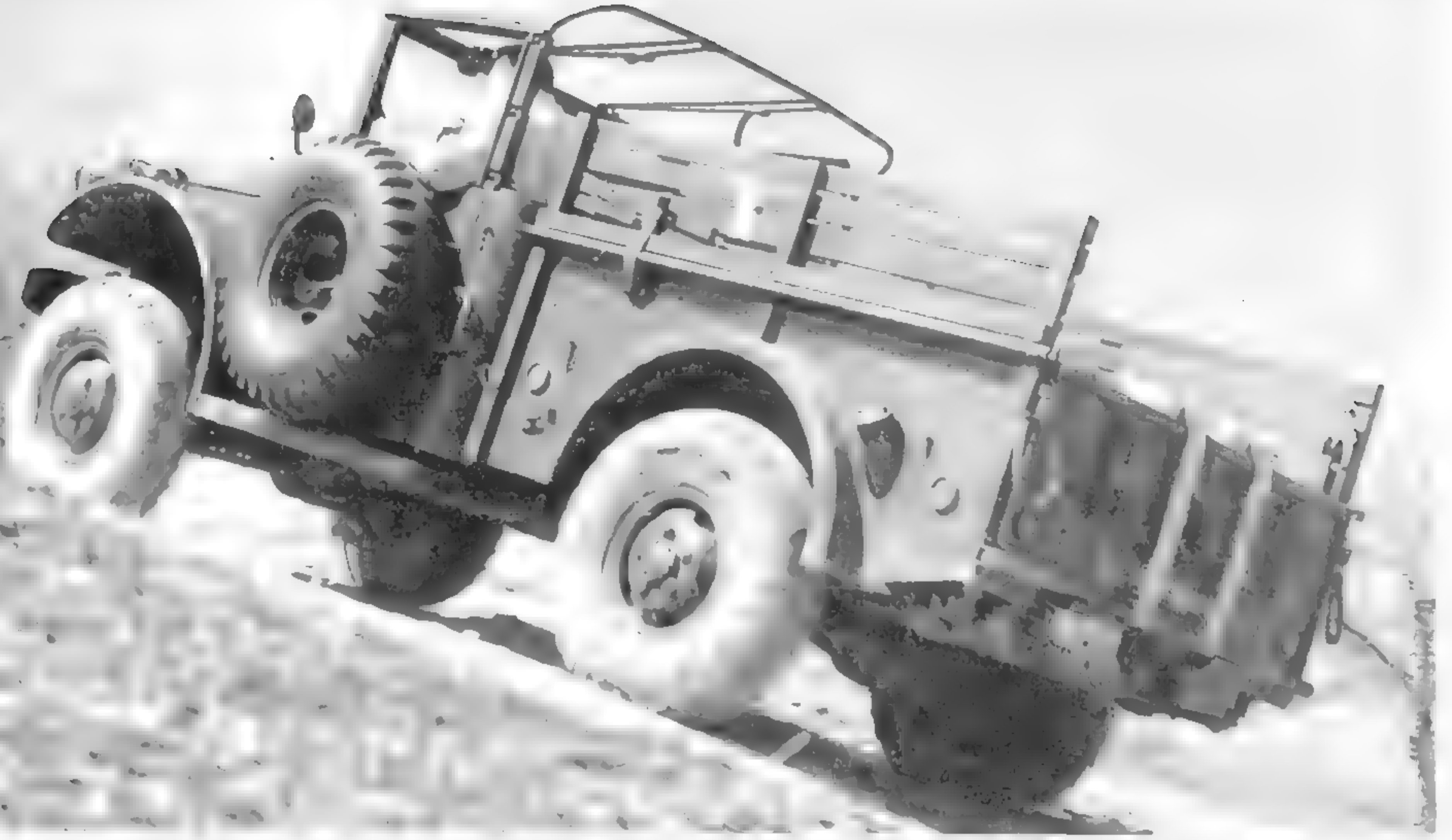
The quickest way to spot an M37B1 is the "door-mounted" spare tire, as seen in this May 1961 photograph. The spare actually was mounted on a hinged rack just outside the driver's door. Previous models mounted the spare tire on the inside front wall of the bed. The passenger-side troop seat was notched to clear it. The other changes characteristic to the B1 vehicles require close examination to spot. (National Archives and Records Administration photo)
